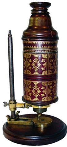
Fig. 1: Microscope used by Robert Hooke Source: https://medicalmuseum.health.mil/micrograph/index.cfm/posts/2019/microscopical_investigation_hookes_microscope ; Public domain: https://commons.wikimedia.org/w/index.php?curid=9583064
